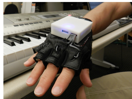
Fig. 1. A PHL glove used in teaching piano melodies.
