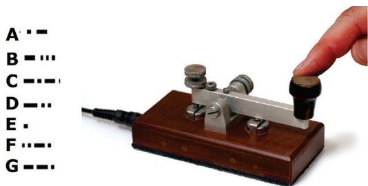
Figure 1. Left: Morse codes for the letters A-G. Right: A straight key for producing Morse.
